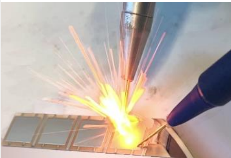
Ignition of electroplated reactive multilayer (Pd-Sn)
