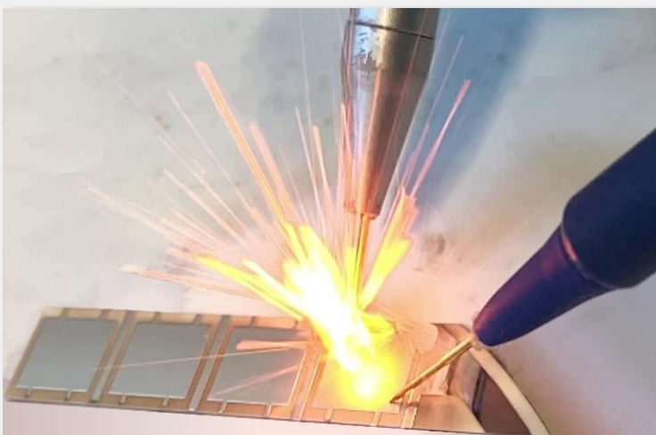
Ignition of Sn/Pd RMS on a ceramic substrate for bond applications.
