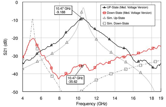
Figure 7. Comparison of the insertion loss between UP- and DOWN-state shows a 25 dB difference.
