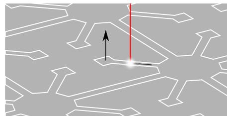
Figure 3. Some elements may be adjusted by local thermal bending
