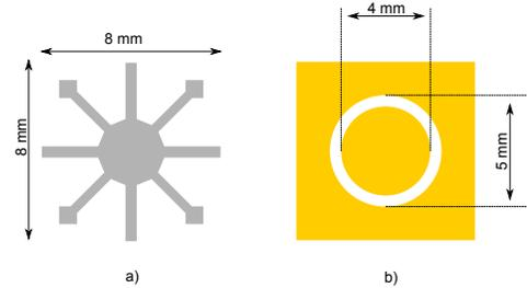
Figure 5. Unit cell of the DC-isolated FSS layers
