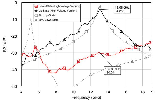
Figure 8. A lower UP-State insertion loss about 4.3 dB was observed for the high-voltage version.
