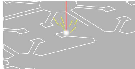
Figure 2. The laser cuts the structure out of a thin metal sheet.
