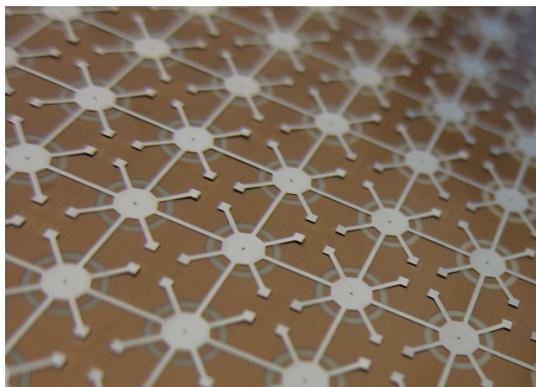
Figure 1. Photograph of the assembled FSS with the cantilevers in UP-State.
