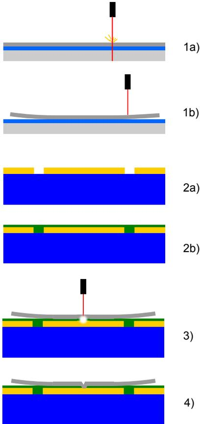
Figure 4. Outline of the laser-machining process flow
