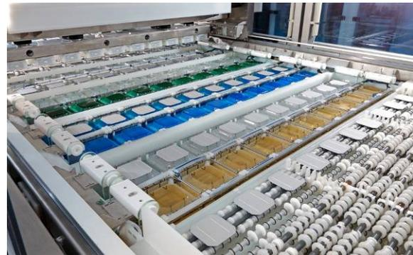
**Fig.4:** RENA CupCellPlate - single side pseudo inline tool for cleaning and Ni/Cu/Sn plating
